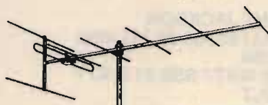
AX-21 1/2 λ - 8 el. Frequenza 136-146 MHz Potenza 200 W Guad. 10 dB Polarizz. or. e vert. Lung. boom mm 2300 Lung. el. max mm 1140
